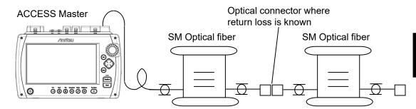
Figure 15.4.1-1 Connection Diagram
