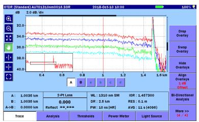
Figure 4.11.2-2 Align Overlays 1 dB Offset
