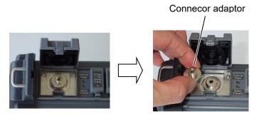
Figure 2.6.2-1 Optical Connector Part
