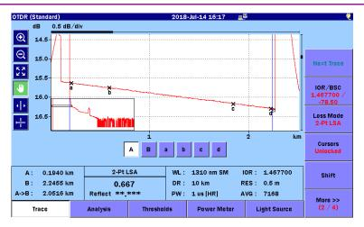
Figure 8.1.2.4-1 2-Pt LSA Measurement Screen
