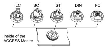
Figure 2.6.2-2 Connector Types
