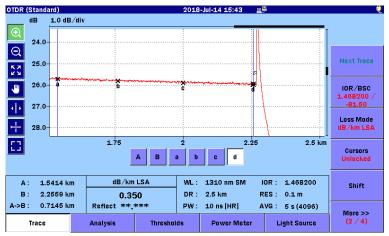
Figure 8.1.2.6-1 dB/km LSA Measurement
