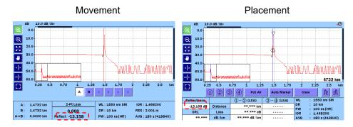
Figure 15.4.1-3 Reflectance Location on the Screen
