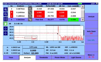
Figure 4.6-1 OTDR (Standard) Analysis Screen
