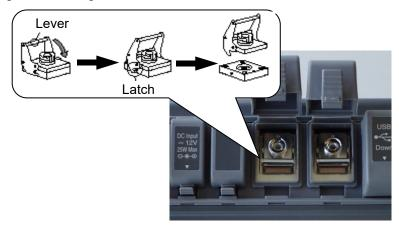
Figure 2.6.1-1 Replaceable Connector
