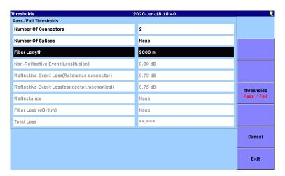
Figure 7.3.5.2-2 Thresholds Screen (Pass/Fail Thresholds, Applicable Standards: ISO/IEC 11801-3:2017)
