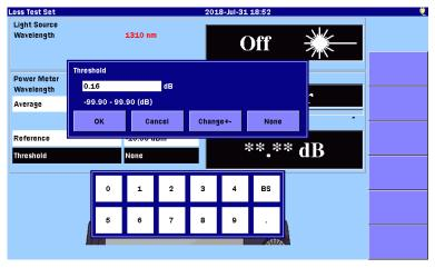
Figure 9.4.2-3 Entering Threshold
