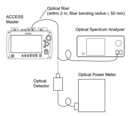
Figure 15.3.8-1 Connection Diagram
