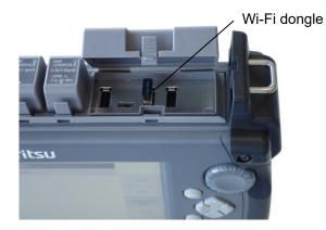
Figure 12.2.2-1 Dongle Connection
