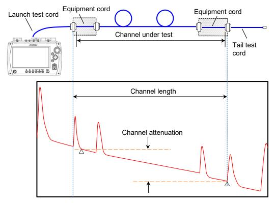
Figure 7.3.2-2 Channel Attenuation
