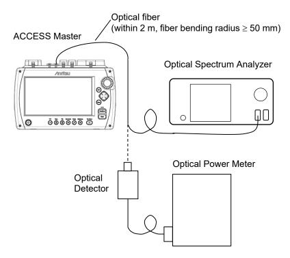
Figure 15.3.7-1 Connection Diagram
