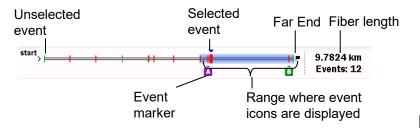
Figure 5.3.1-1 Fiber Schematic
