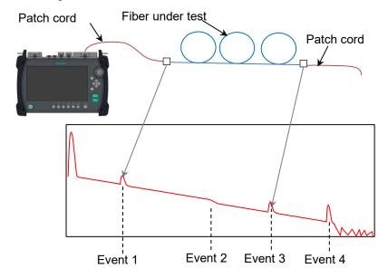
Figure 7.2.3-5 Auto Patch-cord Removal Example
