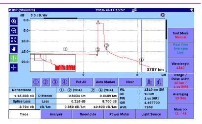
Figure 8.2.3-3 Reflectance Measurements (Points Before and After Reflectance)
