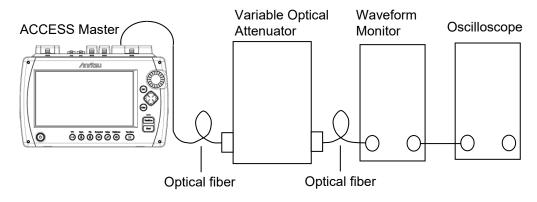
Figure 15.3.2-1 Connection Diagram
