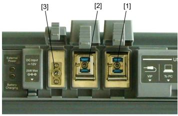
Figure 1 Locations of Laser Beam Apertures
