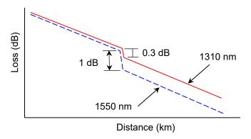
Figure 4.10.1-2 Example of Macro bend Detection
