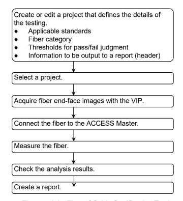
Figure 7.1-1 Flow of Cable Certification Testing
