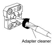
Figure 16.1-2 Cleaning the Ferrule End Surface
