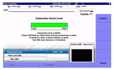
Figure 7.4.1-2 Connection Check Screen
