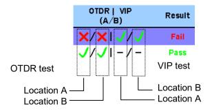
Figure 7.3.9-2 Test Results by Test Location
