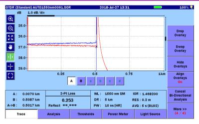
Figure 4.11.3-2 Example of Bi-Directional Analysis Results
