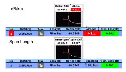
Figure 7.2.3-6 Display of Event Table Span Calculation
