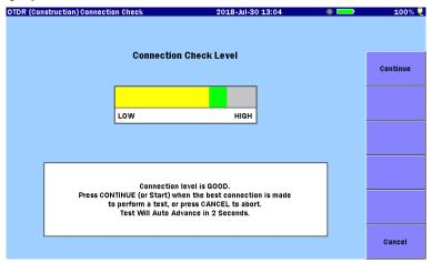
Figure 6.5-1 Connection Check Screen
