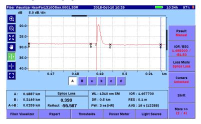
Figure 5.6.1-4 Fiber Visualizer Trace Screen (Manual)
