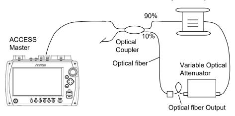
Figure 15.3.6-1 Connection Diagram
