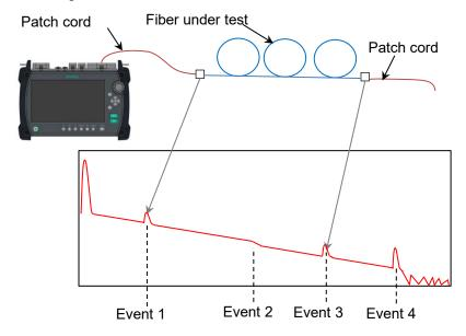
Figure 5.2.3-5 Auto Patch-cord Removal Example
