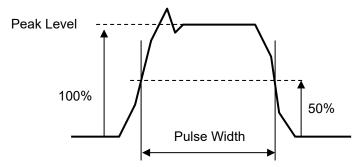
Figure 15.3.2-2 Pulse Width Measurement
