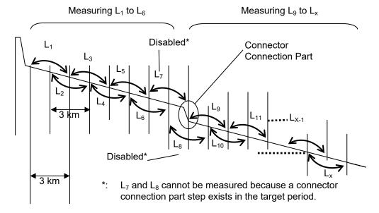
Figure 15.3.5-2 How to Measure Linearity
