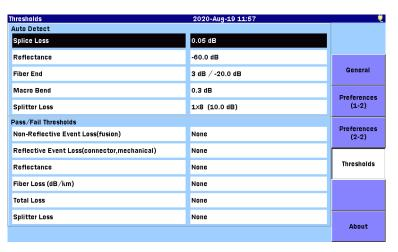
Figure 6.2.4-1 Thresholds Screen
