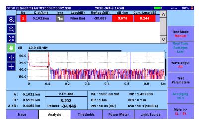
Figure 4.10.2-1 Analysis Screen for All Wavelengths
