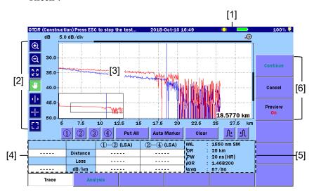
Figure 6.5-2 Test In Progress Screen
