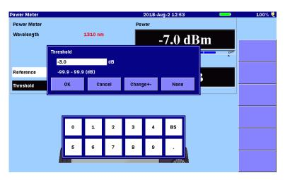
Figure 10.3.3-1 Entering Threshold
