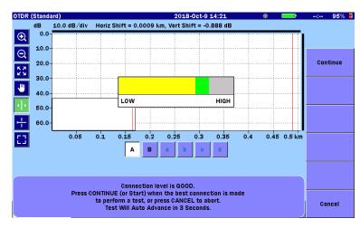
Figure 4.5.6-1 Connection Check Screen
