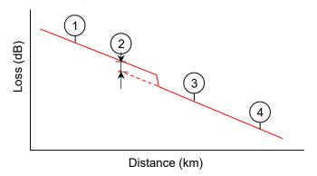
Figure 4.5.5-2 Splice Loss
