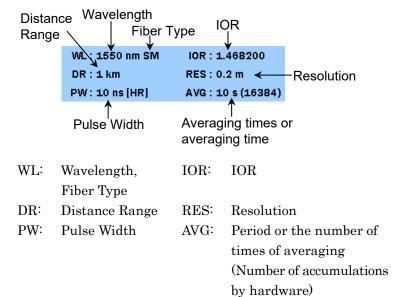
Test parameters for the primary trace are displayed for a trace recalled from a file.
