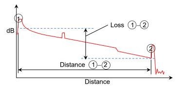
Figure 8.2.1-1 Distance and Loss Measurement between Two Points
