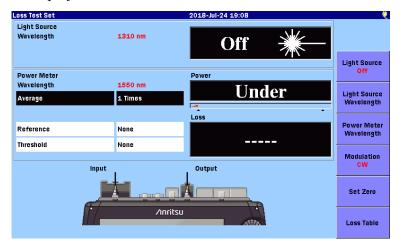
Figure 9.2-1 Initial Loss Test Set Screen
