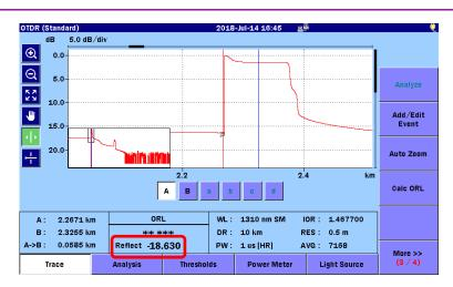
Figure 8.1.3.2-2 Manual Reflectance Calculation Screen
