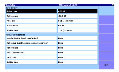
Figure 4.2.7-1 Thresholds Screen
