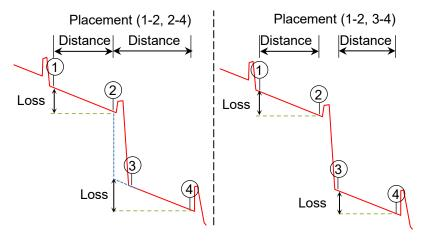
Figure 7.2.3-4 Display of Distance and Loss Between Markers
