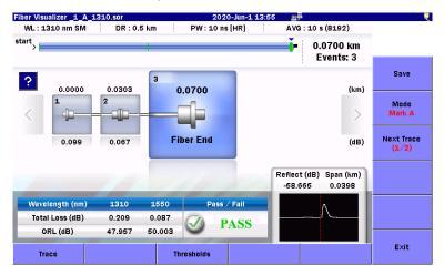
Figure 7.4.1-4 OTDR Test Results
