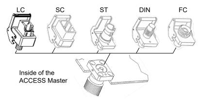
Figure 2.6.1-2 Connector Types
