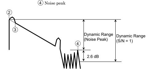
Figure 15.3.3-2 How to Measure Dynamic Range
