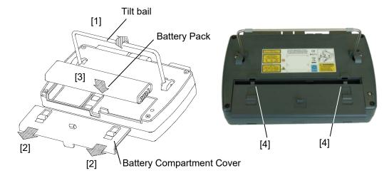
Figure 2.2.1-1 Installing the Battery Pack
