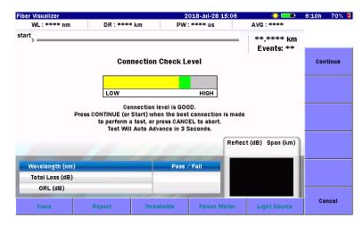
Figure 5.4.1-1 Connection Check Screen
