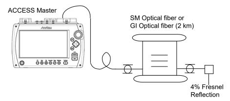
Figure 15.3.4-1 Connection Diagram
