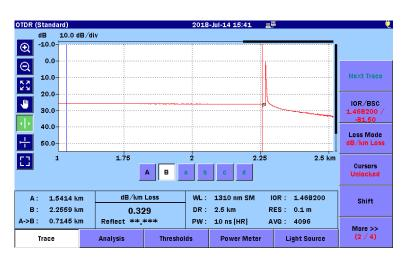
Figure 8.1.2.5-1 dB/km Loss Measurement Screen
