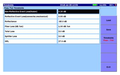
Figure 5.2.6.2-1 Thresholds Screen (Pass/Fail Thresholds)
