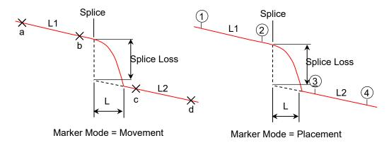
Figure B.2-2 Measurement Principle of Splice Loss
