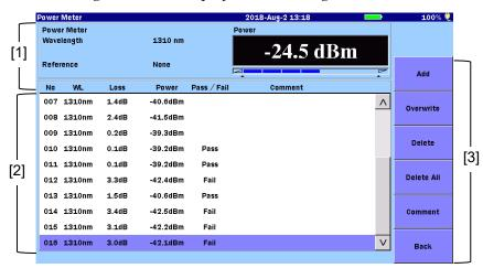
Figure 10.2-1 Loss Table Screen (Power Meter)
