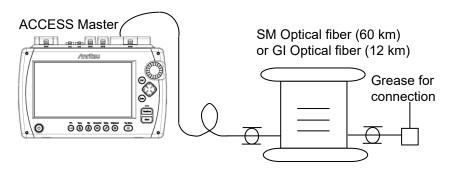
Figure 15.3.5-1 Connection Diagram
