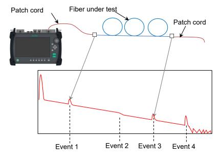
Figure 4.2.3-5 Auto Patch-cord Removal Example
