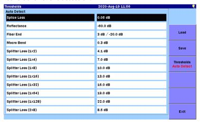
Figure 5.2.6.1-1 Thresholds Screen (Auto Detect)
