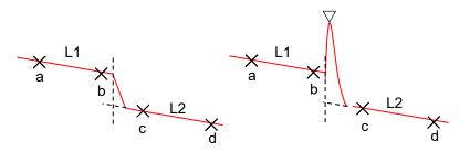
Figure B.1-1 Method to Obtain Splice Loss (Marker Mode = Movement)
