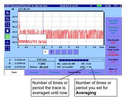
Figure 4.4-1 OTDR (Standard) Mode Screen—Measurement In Progress
