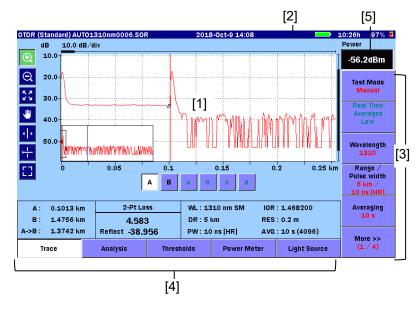
Figure 4.5-1 OTDR (Standard) Trace Screen
