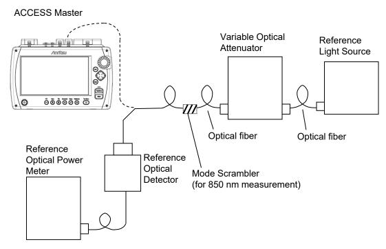
Figure 15.3.9-1 Connection Diagram
