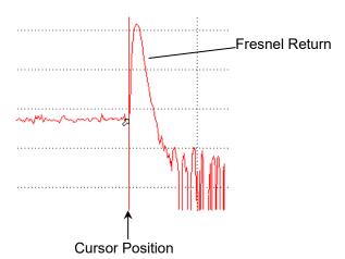
Figure 15.3.4-2 Cursor Placement for Distance Measurement Accuracy Test
