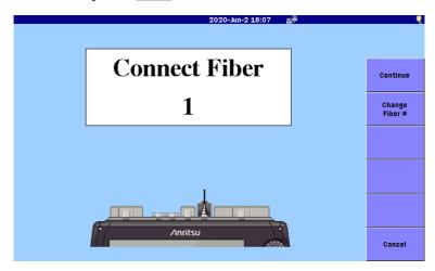
6. When, in "**Preferences (1–2)**", **Connection Check** is set to **On**, the Connection Check Level screen appears. Touch the **Continue** softkey. When the connection status is good (green), the process proceeds to step 7 automatically in 3 seconds.
