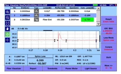
Touch the **Result** softkey (on softkey page 2) and display **Manual** on it, and you can see the enlarged view of the trace graph.
