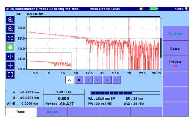
4. When **Preview** is On, after the analysis after measurement is completed, the Summary dialog box is displayed. Touch **Close** to check waveform.
