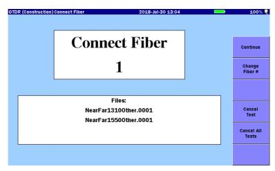
3. Connect the fiber under test to the ACCESS Master and touch **Continue** to start a measurement. To confirm test results when the measurement finishes, touch **Preview** to turn it On.
