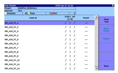
4. Touch **Start Test** or press **Start**. Touch **OTDR** or **VIP**. For how operate to the VIP, refer to page 48.
