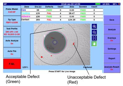
If the size of a defect found on the fiber endface is acceptable, the defect is highlighted in green. If the size of a defect found on the fiber endface is unacceptable, the defect is highlighted in red.
