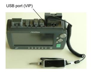
When the VIP is connected to the ACCESS Master, touching  $\overline{\text{VIP}}$  on Top Menu displays the VIP screen.
