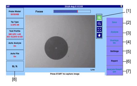
The **Focus** bar indicates the degree of the focus adjustment.
