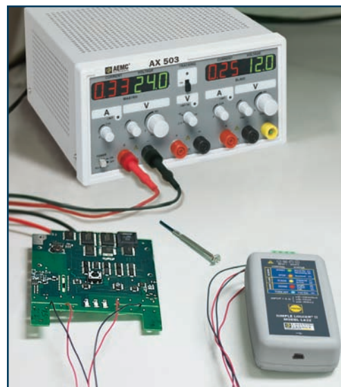
L432 recording two DC voltage supplies.
