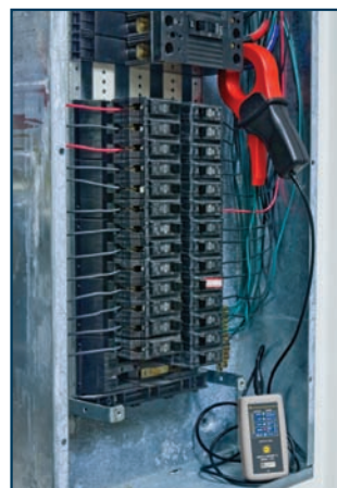
L101 recording branch circuit current.
