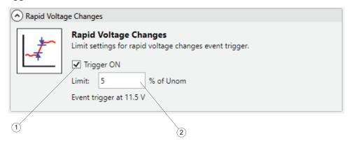
To enable the RVC trigger, select the **Trigger ON** check box (1). A Rapid Voltage Change event is triggered, if the difference between two steady states exceeds the trigger threshold. The Logger captures the event along with detailed data. Disable the trigger to save Logger memory if not needed.
