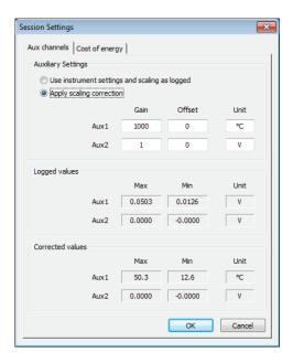
Click **OK** when the "Corrected values" are as expected. Energy Analyze Plus now shows the corrected scaling of values.
