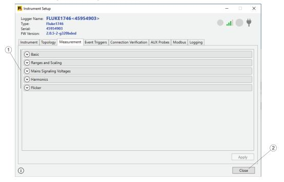
Content of the Measurement tab depends on the capabilities of the Fluke Logger you are about to configure. Features not supported by a Logger are not shown. See the users manual for the Logger for details on supported features.
