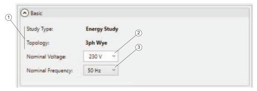
The Nominal Voltage selector ② lets you select the nominal voltage of the grid from a list of common settings in low-voltage nets. You can enter a custom setting if the list does not contain the correct setting. The definition of event triggers will depend on this setting.
