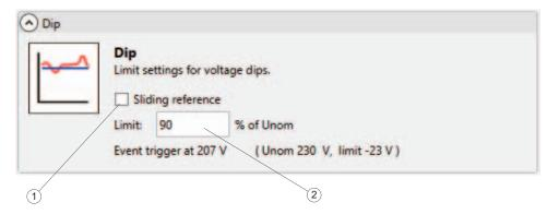
Disable **Sliding reference** mode to apply a fixed voltage level for triggering Dip events.
