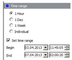
A time range is set with the controls located under the Graph Options at the right-hand side of a graph screen. Use the radio buttons to quickly adjust the time-axis to contain the selected time span.
