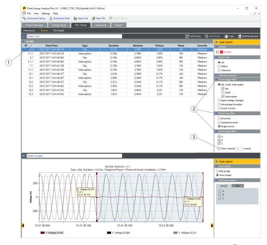
Click on a table header cell to sort the entire table. A small triangle (1) to the right of the table header cell marks the sorting parameter and the ascending or descending sequence of the list. Use the Event filter elements (2) to optimize long lists of event records. Also, an option to limit the number of list entries (3) is available in this view. You cannot add notes to this view.
