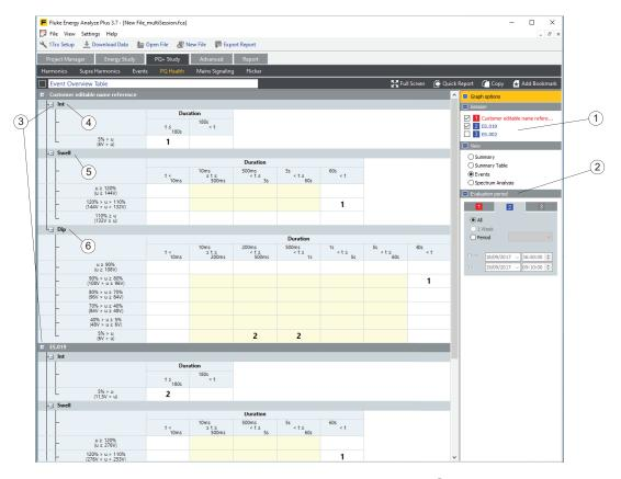
If more than one session is loaded, these list as sources ① in Graph Options. Each has a check box that enables or disables a corresponding table section. Table sections expand or collapse with the blue icons ③ on the table headers.
