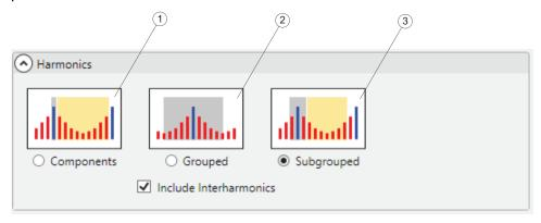
To log Grouped Components, select the **Grouped** (2) model. Average signal levels of frequency bins that lie between harmonic frequencies will be distributed between two harmonic bins. That is, half of frequency bins including interharmonics (red bars,
