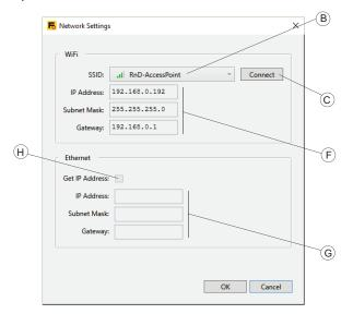
To configure the Logger to connect to a WiFi access point, select from the options in the SSID box. The setup tool requests a list of discoverable SSIDs from the Logger and offers the result, along with associated field strength, as options. Select the SSID (B). If the access point to connect to works with a hidden SSID, select that entry. Click **Connect** (C).
