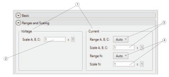
To adjust the scaling of voltages for use with voltage transducers, make sure to have configured the Nominal Voltage in the Basic Settings section to the reading of the primary side of the voltage transducer. Then enter the transducer-ratio in the Voltage Scaling text box ②. This setting affects the definition of Event triggers.
