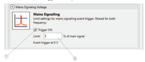
Enter a Limit value (2) relative to the adjusted Nominal Voltage to define the trigger threshold. Disable the trigger to save Logger memory if not needed.
