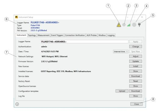
The panel shows the Logger state 6, lets you view and change settings on the Logger 7, and contains buttons 8 that let you apply changes or exit configuration. Status information contains the Logger name, serial number, and the firmware revision. Icons provide further detail:
