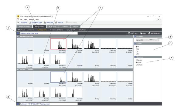
Calendar View  $\bigcirc{2}$  helps to quickly identify change patterns in parameters and lets you compare these changes by parameter in detail.
