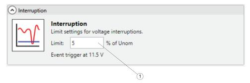
A voltage Interruption event is triggered if the level of all half-cycle RMS voltage channels goes below the defined threshold. See the users manual for the Logger for more detail on Interruption events.
