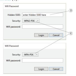
Depending on the configuration of the access point you chose, setup tool will ask for a passphrase – enter the passphrase of the WiFi Access Point. The setup tool will pre-select the security algorithm (E) based on the published capabilities of a discovered network (SSID).
