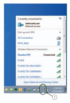
4. Select the Logger to connect to, compare the listed SSIDs with that shown on the WiFi Configuration page (for more information, see the users manual for the Logger), and chose the matching one.
