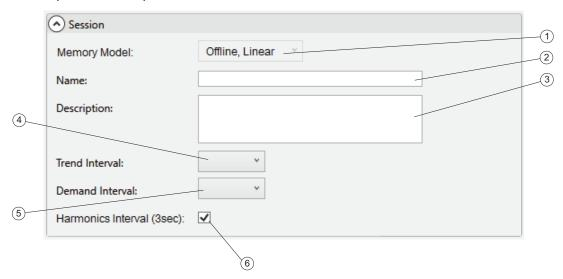
If you select a linear model, the Logger logs until the defined end date is reached and then stops.
