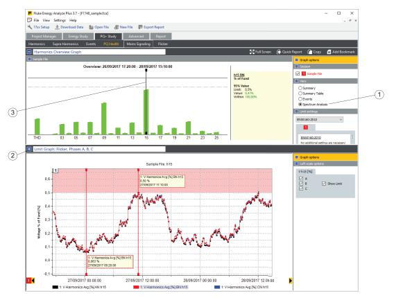
Select a standard 1 and Energy Analyze applies the limits to the measured data according to the standard. You can directly navigate to detail views 2 by selecting a bar 3 of specific interest.
