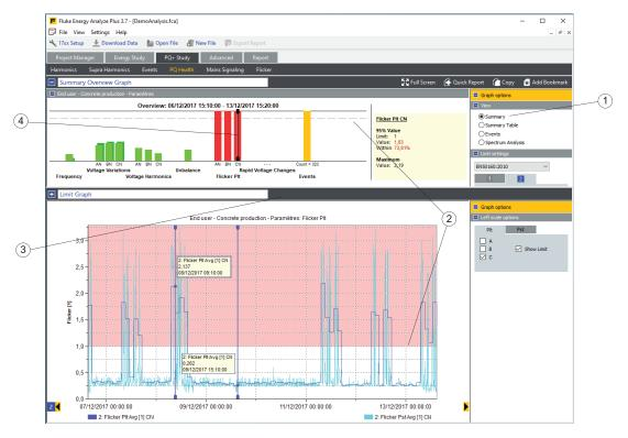
The example above shows an evaluation that complies with EN50160. For each mandatory parameter, a bar represents the proximity to the relevant limit. The Voltage Harmonic bars represent groups of parameters. The length of the bar is determined by the worst condition for the entire group. Position the cursor on a bar in the "Summary Overview Graph" to get more detail. See "Limit Graph".
