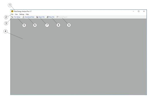
When started from the Windows Start button, Energy Analyze Plus does not automatically load data – the main window title  $\bigcirc$ 1 shows the software name and version, the menus  $\bigcirc$ 2, and the toolbar  $\bigcirc$ 3. The main panel  $\bigcirc$ 4 is empty.
