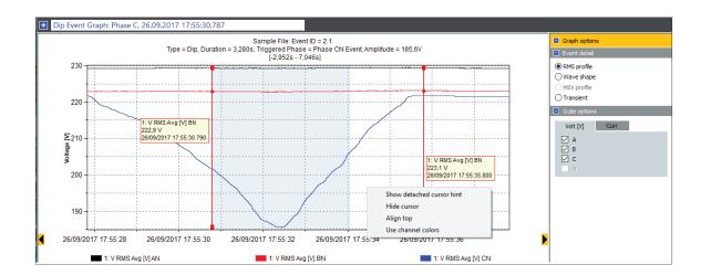
**Show detached cursor hint** moves the cursor text fields out of the graph area to the top or to the right of the chart. In detached mode, a delta function shows the difference in data between cursor 1 and cursor 2.
