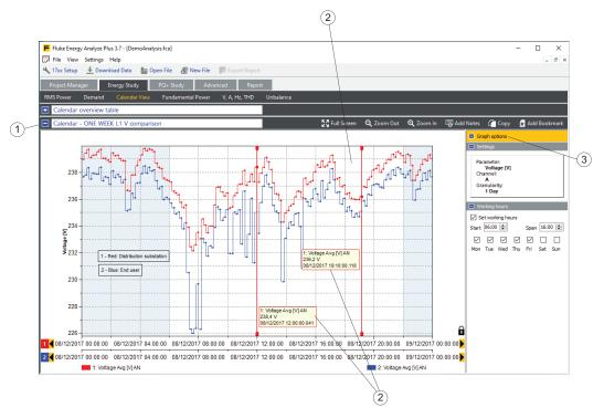
A detail plot (2) of the data selected in the overview table shows in the graph section (1). Information about the plot traces is found in the "Graph Options" (3). As in other graph views, use the vertical cursors to get numerical readings of data "behind" curve points (4).
