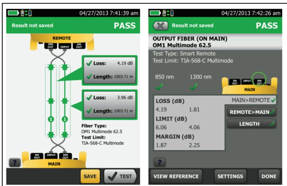
Figure 4. Examples of Fiber Test Results Screens
