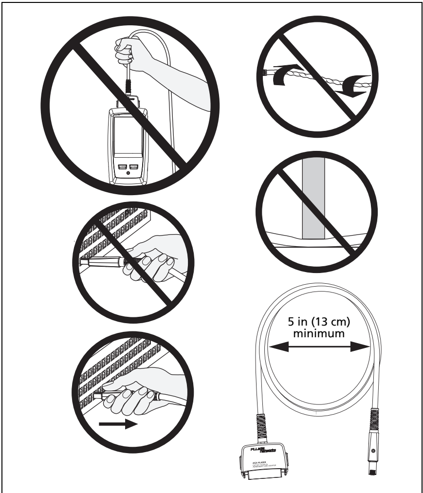
Figure 4. How to Prevent Damage to the Permanent Link Adapter Cables
