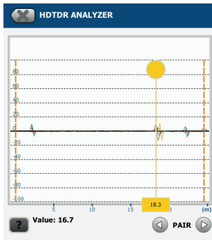
③ Bad patch cord
