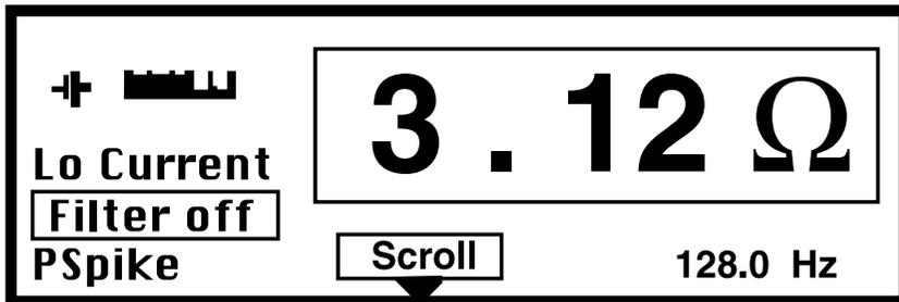
3. If required, carry out a **Pspike** test to check continuity of the the Potential circuit.
