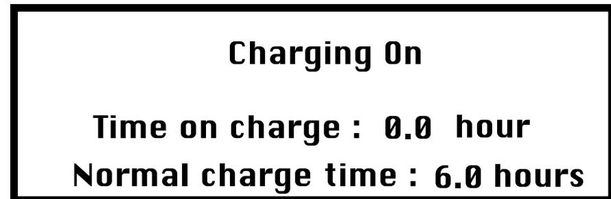
5. When fully charged, the charging current will automatically reduce to "**Trickle Charge**". Charging will automatically stop after a period of 24 hours.
