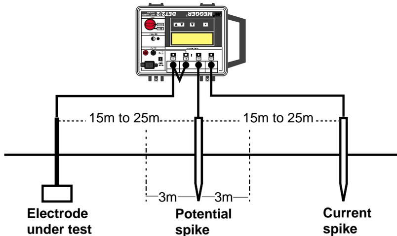
**Fall-of-Potential method using a single lead to the earth electrode.**
