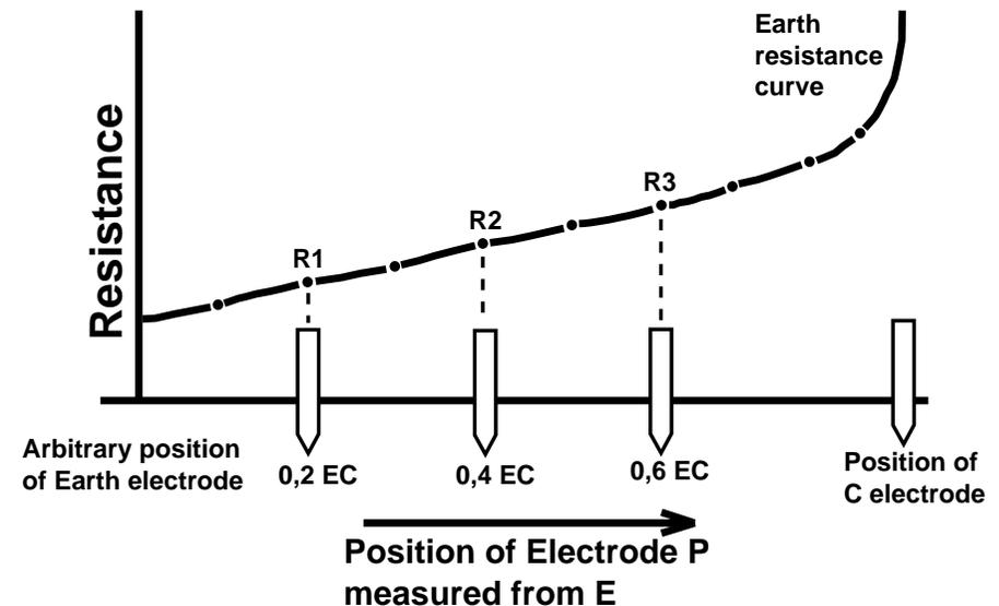
**Example Resistance curve from Slope method tests.**
