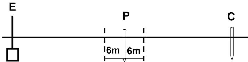
Test spike positions for BS7671 testing
